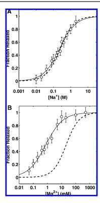
**Figure 3.** Ion-mediated structural relaxation fit to the empirical Hill model for Na<sup>+</sup> (A) and Mg<sup>2+</sup> (B). Fraction relaxed reflects the overall relaxation of the ensemble as determined by projection onto the experimental scattering profiles taken at low- and high-ionic concentration (see eq 1). For both plots, solid lines show the Hill fit to the experimental data and the dashed lines show the same relaxation derived from PB.
